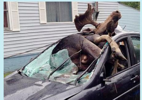
active from dusk to dawn, when their coloration makes them difficult to see in the roadway and their eyes are usually above the reach of car headlights. Moose are so tall that an automobile usually passes under the body, causing the moose to come over the hood into the windshield and onto the roof.
